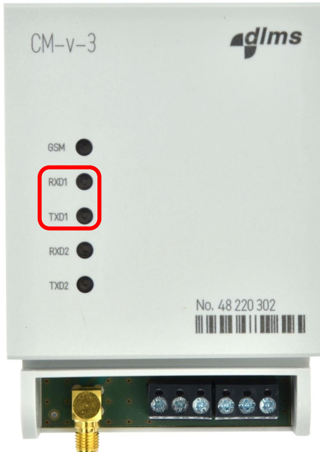
Figure 4: Primary communication channel LEDs position on the front plate
