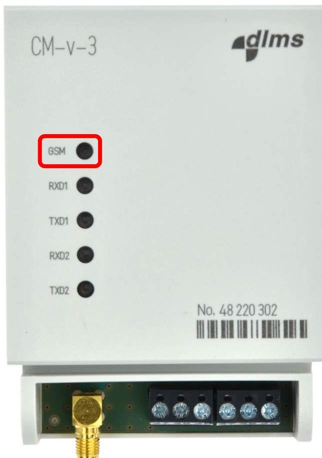
Figure 3: GSM LED position on the front plate
