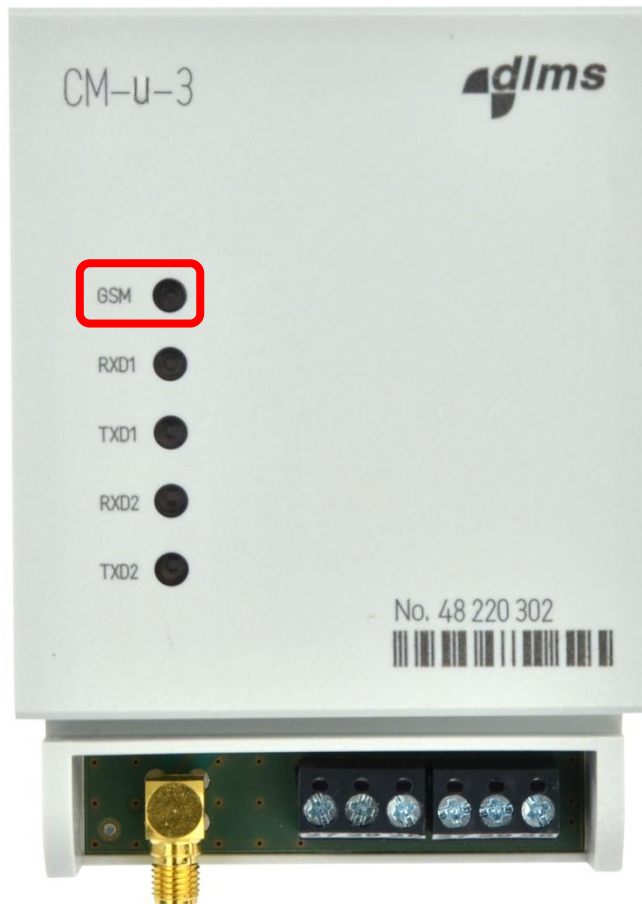
Figure 3: GSM LED position on the front plate
